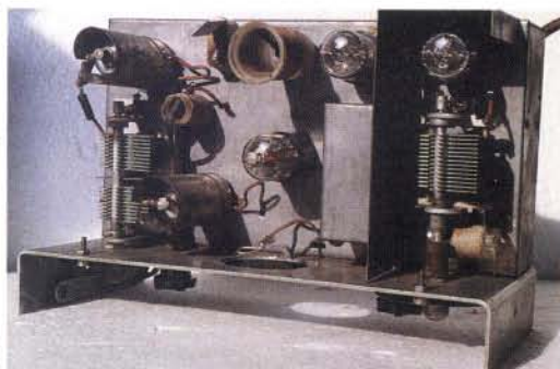
Fig. 7: Inside the Teco set with the receiver on the left, transmitter on the right. The modulator is in the centre and the p.a. stage tank coil at the top centre.
