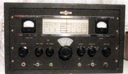
Fig. 2: The Collins 32V-1 transmitter clearly illustrating its very finely engineered tuning dial arrangement and symmetrical dial layout (see text).
